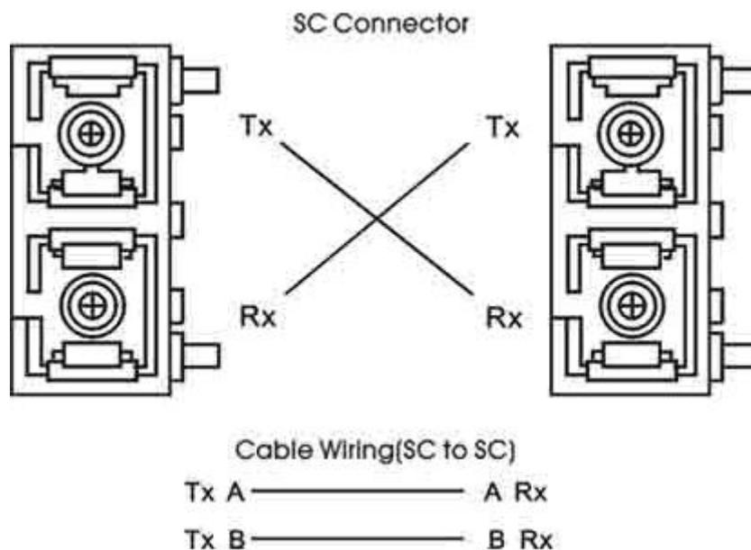
Fig. 7: Connecting the Fiber Ports
