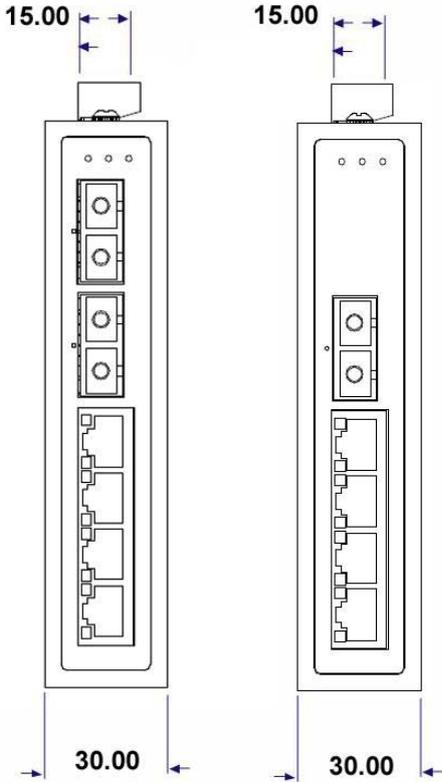
Figure 2a: Front View of 4 10/100TX + 1x or 2x 100FX Industrial Switch
