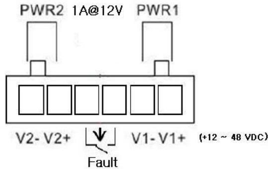
Fig. 6: Pin out Power Connector and Alarm Contact
