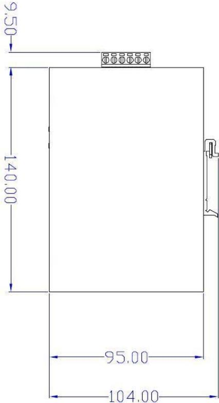
Figure 2b: Side View of 4 10/100TX + 1x or 2x 100FX Industrial Switch
