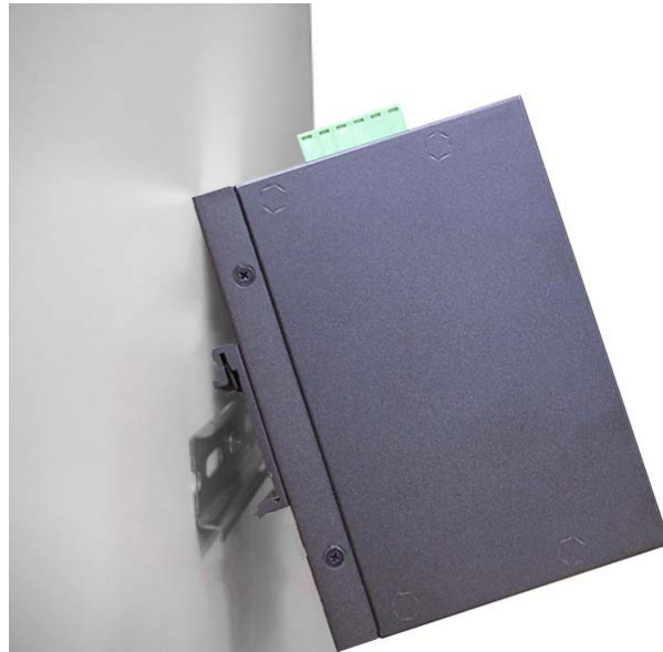
Fig. 3: Installation to DIN-Rail Step 1
