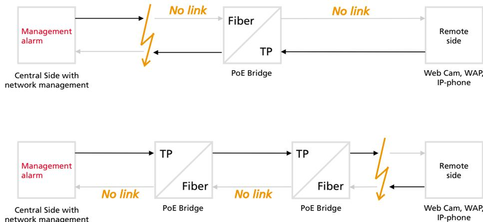
Link Through function only takes effect when switch 4 is activated.
