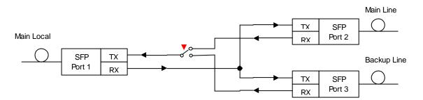
Port 1 is the local port, port 2 is the main connection and via port 3 the backup line will be connected. In this mode the port 4 will not be used.
