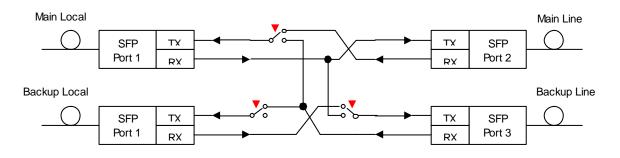
As opposed to the "normal protection mode" the fourth port will be used with in the mode "protection with load rejection".
